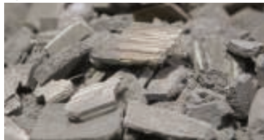
FIGURE 2. Spent automotive catalysts contain valuable precious metals, such as palladium, platinum and rhodium
