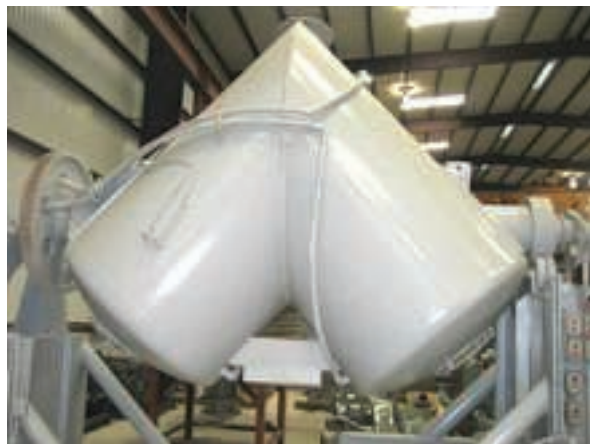
FIGURE 3: Traditional blenders can be modified to be used as vacuum dryers (Source Patterson Kelley)
