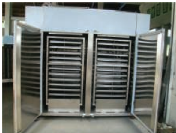
FIGURE 2: Vacuum tray dryers are common for laboratory and pilot-scale work
