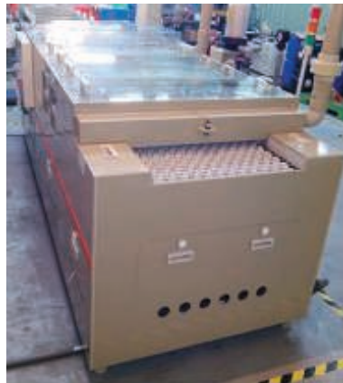
FIGURE 5. Automatic gold-stripping machines allow for efficient treatment of printed circuit boards
